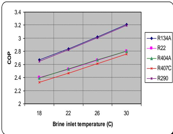
Figure 7: Variation of first law efficiency in terms of coefficient of performance (COP) vs. Brine inlet temperature of different ecofriendly refrigerants
