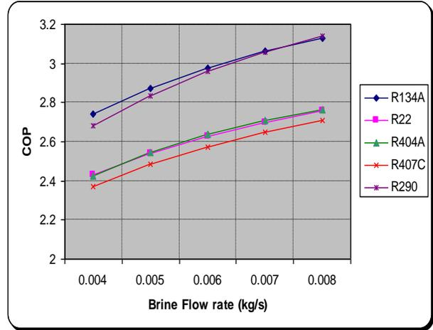
Figure 4: Variation of first law efficiency in terms of coefficient of performance (COP) vs. Brine flow rate of different ecofriendly refrigerants
