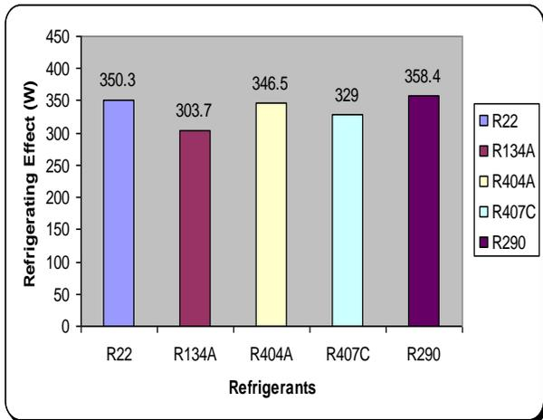
Figure 3: Comparison of refrigerating effect of different ecofriendly refrigerants
