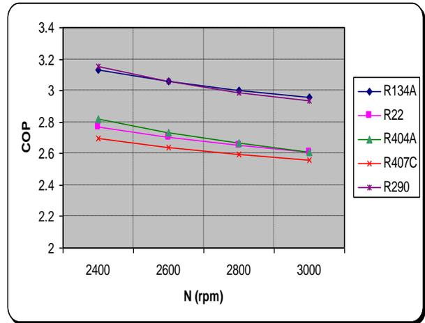
Figure 8: Variation of first law efficiency in terms of coefficient of performance (COP) with speed of compressor of different ecofriendly refrigerants
