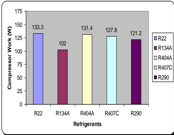
Figure 2: Comparison of compressor work of different ecofriendly refrigerants
