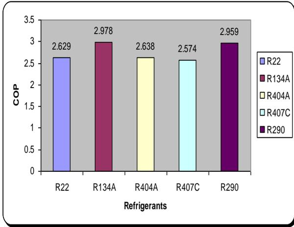
Figure 1: Comparison of COP of different ecofriendly refrigerants
